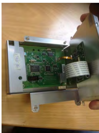
Communication between touch screen and display PCB
