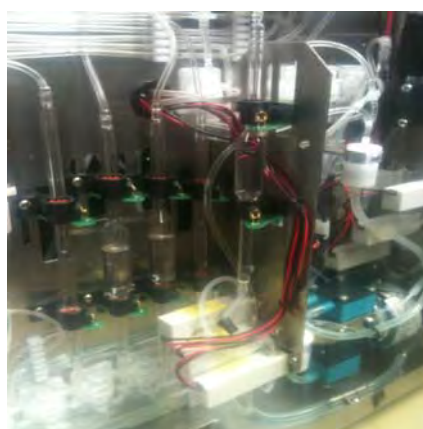
Figure 2.32 Eos pipette with extra inlet valves
