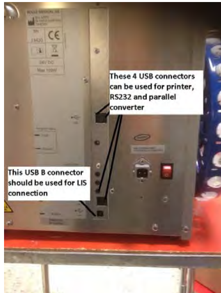
CPU board with only USB ports (1091373_S CPU board Human) (1091394_S CPU board Vet)
