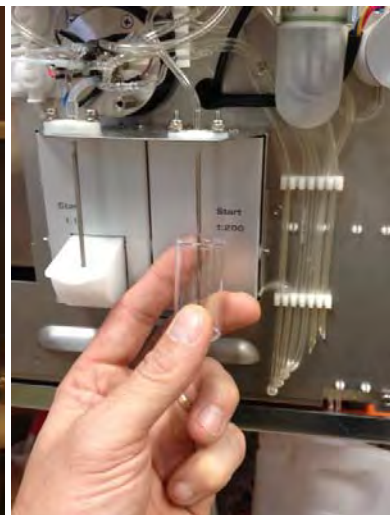
Aspirate Hypochlorite through predilute
